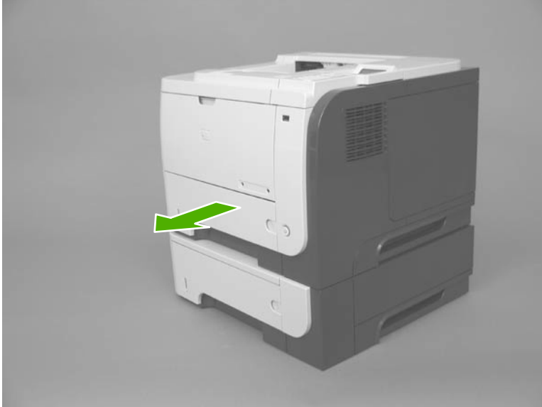
Figure 2-6 Remove the tray cassette (1 of 2)
