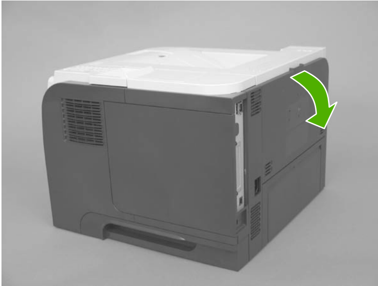
Figure 2-20 Remove the rear-door assembly (1 of 8)
