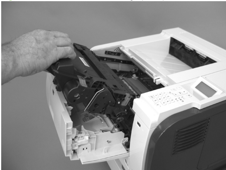
Figure 2-5 Remove the toner cartridge (2 of 2)
