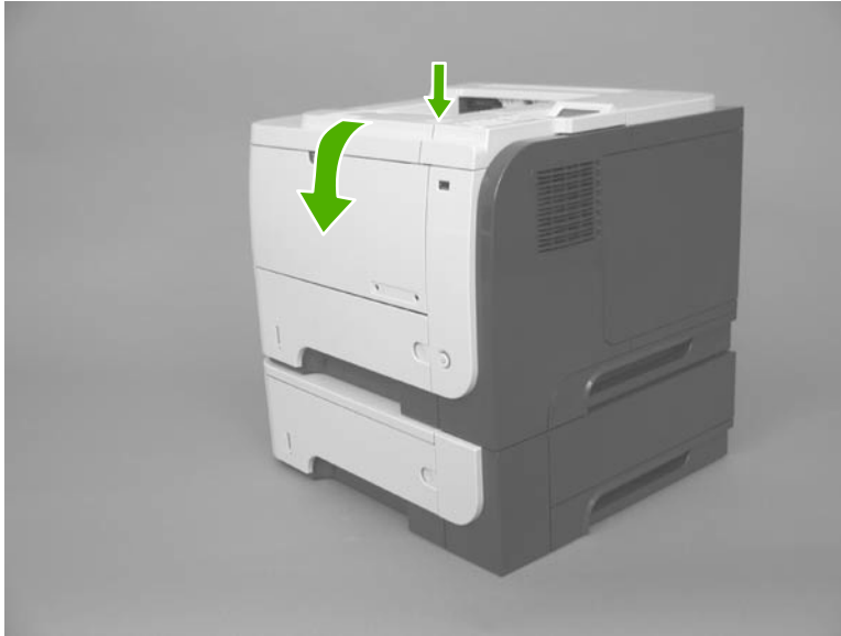
Figure 2-4 Remove the toner cartridge (1 of 2)
