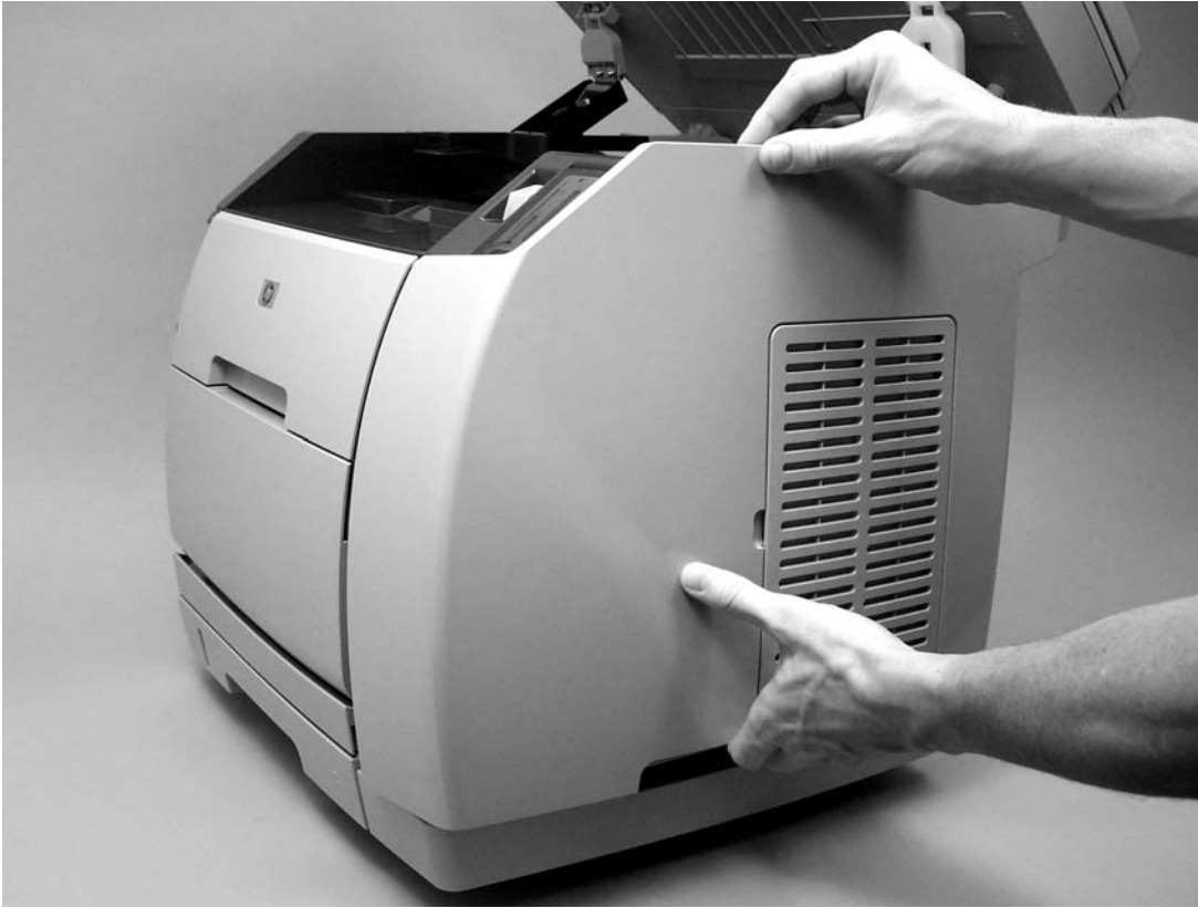
Figure 5-24 Remove the right-side cover (2 of 2)
