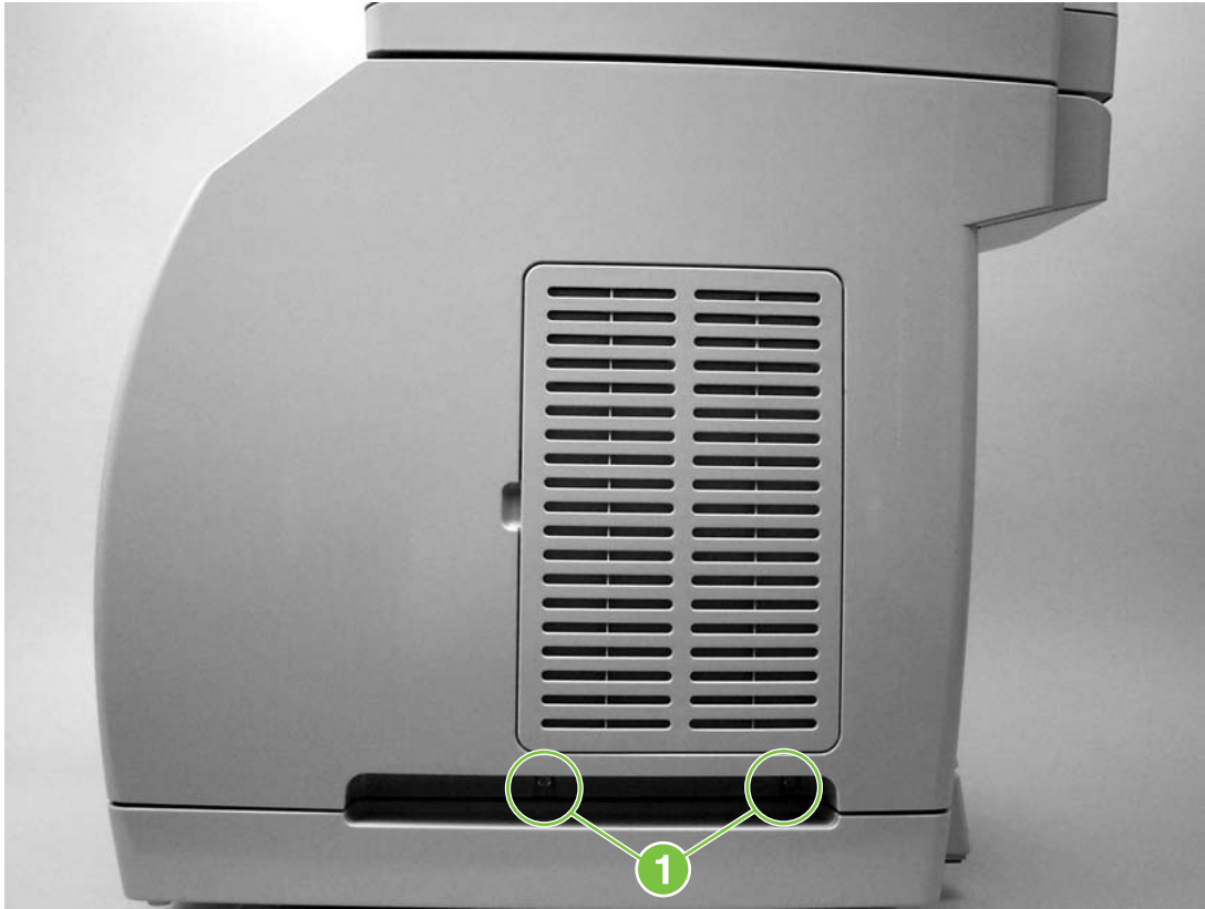
Figure 5-23 Remove the right-side cover (1 of 2)
